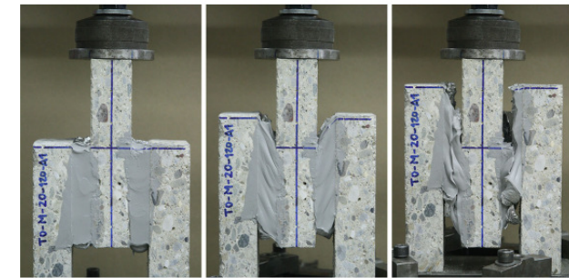
Monotonic testing on assembled specimen
