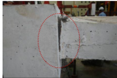
Welding Broken between Headed Stud Steel Anchor and Steel Plate
